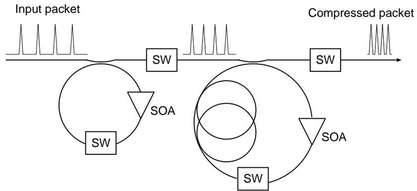
Fig. 1. Optical packet compressor
