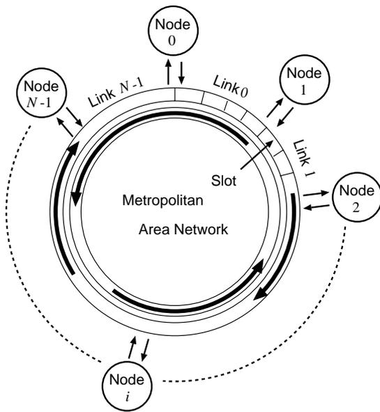
Fig. 2. A bidirectional ring with optical compression TDM
