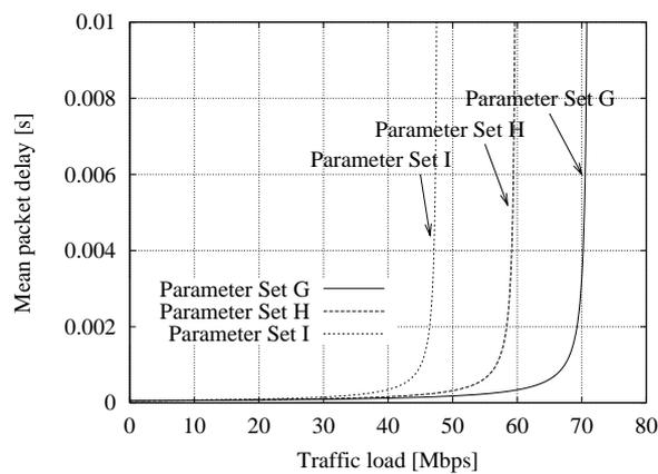
Fig. 17. The packet delay time for parameter sets G, H and I
