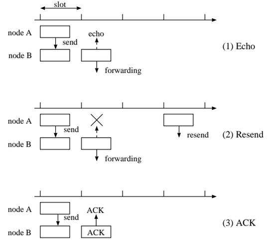
Figure 2: Time chart of packet transmission
