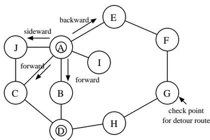
Figure 3: Selection of route for retransmission
