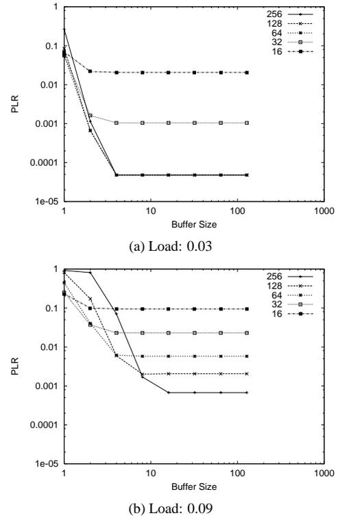
Figure 6: Estimation of sufficient buffer size
