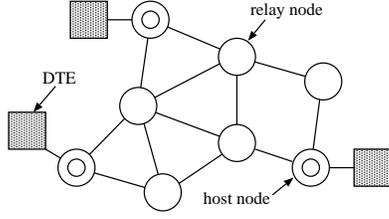
Figure 1: Components of Flexible Radio Network
