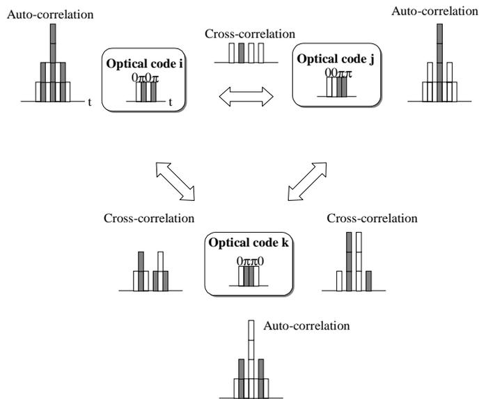
Fig.7 Optical correlation between two optical codes
