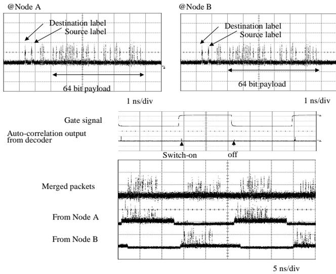
Fig.13 Measured waveforms; generated 64-bit long packets with two photonic labels in the header (on the top), generated control signals (in the middle), and the merged and split packets (on the bottom)
