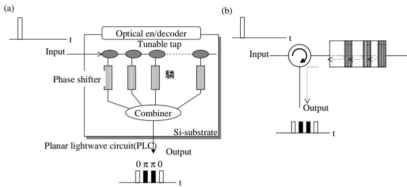
Fig.8 Optical encoder / correlator: (a) Waveguide tapped delay line and (b) FBG
