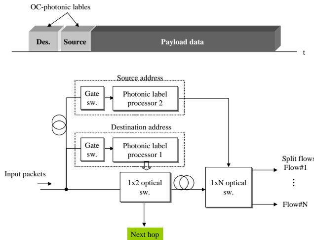
Fig.6 Architecture of photonic label processor which performs split of the flows
