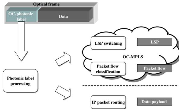
Fig.2 Basic idea using OC-photonic labels as the identifier of LSP, IP packet, and packet flow
