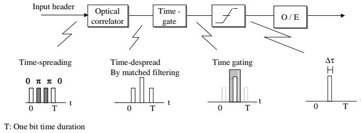
Fig.9 Block diagram of photonic label processor
