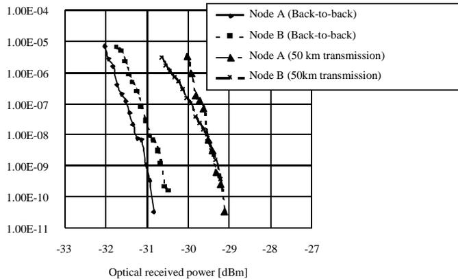
Fig.14 Measured bit error rates (BERs) vs optical received power
