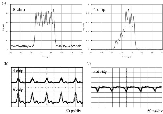
Fig.11 (a) Optically-gated control codes, (b) optical decoder outputs: auto-correlation waveforms, and (c) output of a dual-pin PD
