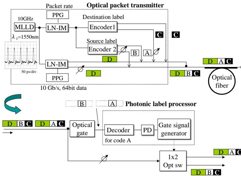
Fig.12 Experimental setup for photonic split of merged flowS
