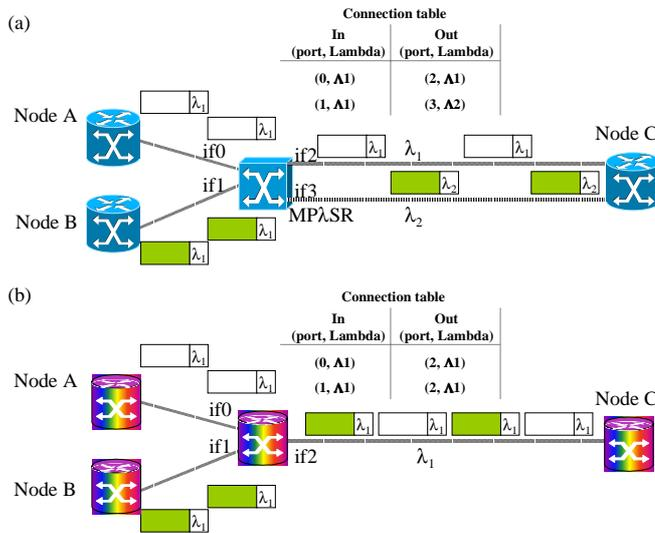
Fig.5 Classification of packet flow in (a) MPLS network and (b) OC-MPLS network
