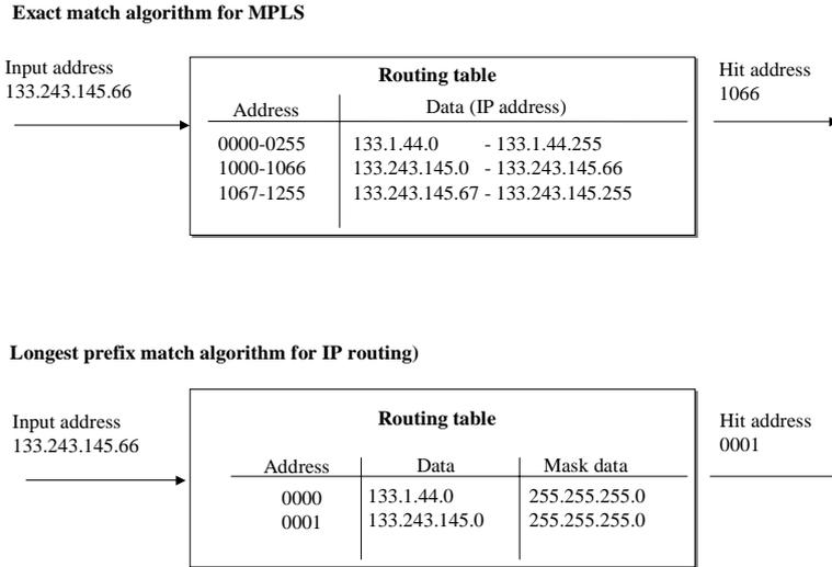
Fig.3 Forwarding algorithms : Longest prefix match and exact match
