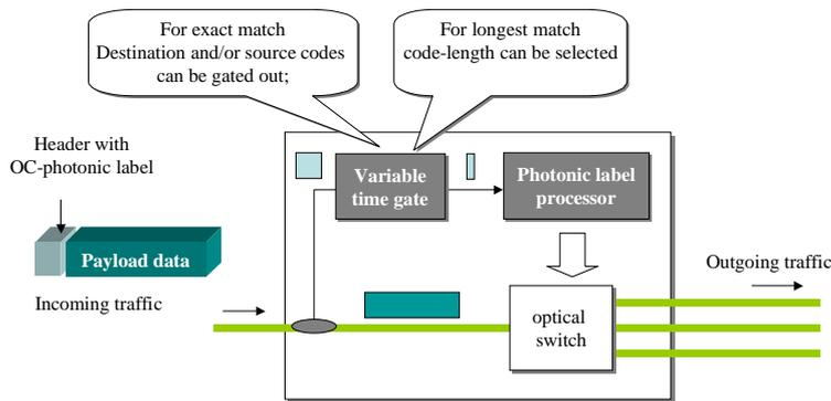
Fig.4 Architecture of OC-photonic label processor for exact match and longest match
