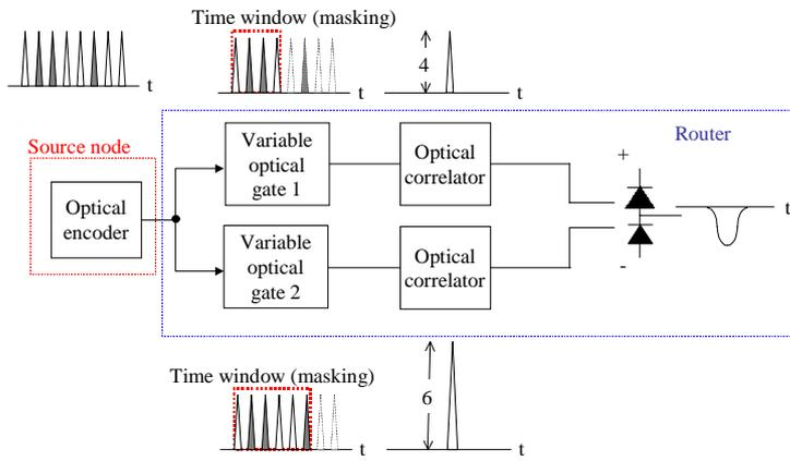
Fig.10 Experimental setup for longest prefix match
