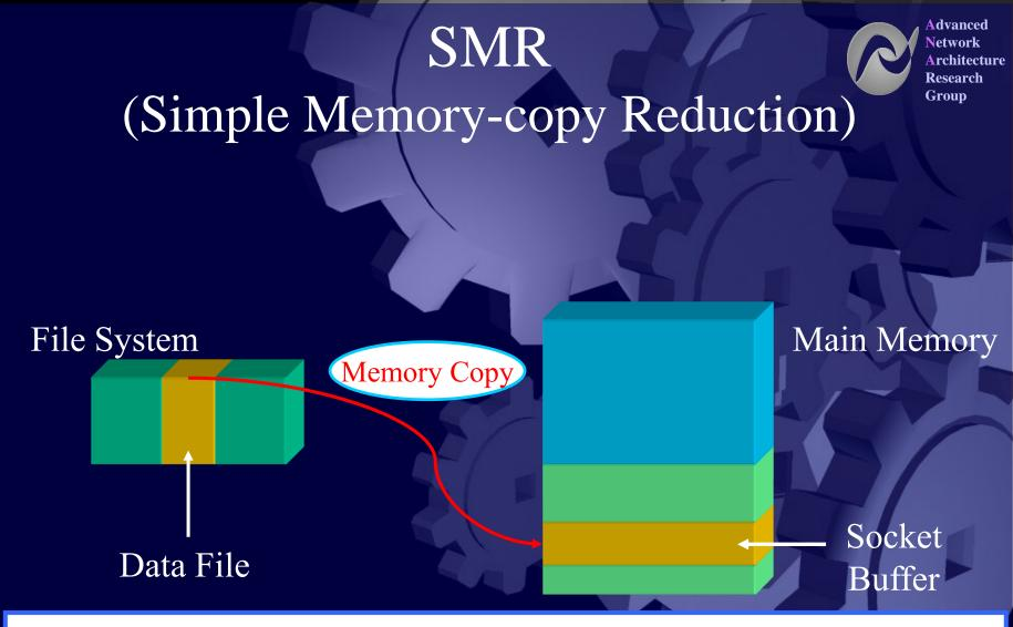
SMR scheme reduces the data transfer overhead at the sender host by reducing the redundant memory copy operations
