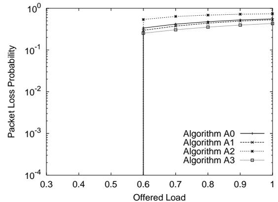
Figure 8: Packet loss probability (shared buffer type switch, for  $B = 64$ )
