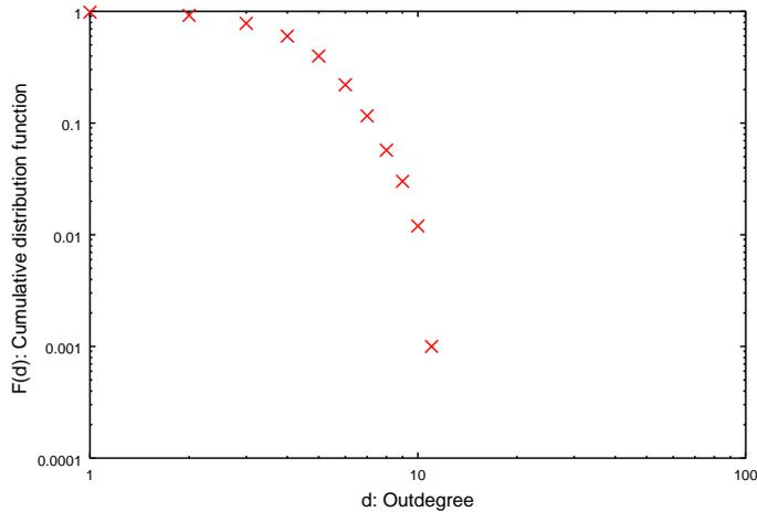
Figure 4: Cumulative distribution function of outdegrees in a topology generated with the ER model
