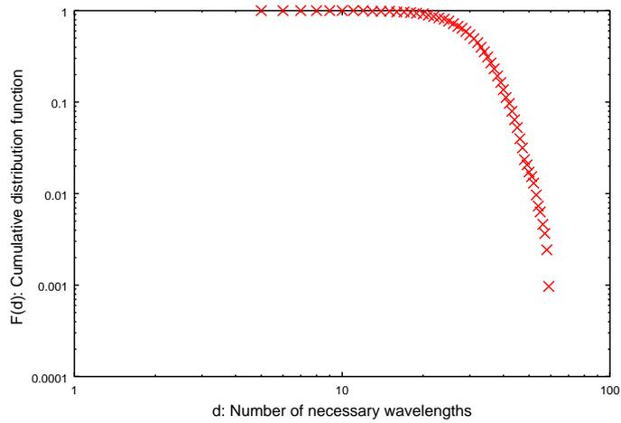
Figure 10: Distribution of the number of required wavelengths: the ER model without wavelength conversion
