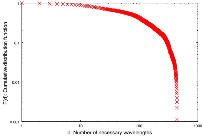
Figure 8: Distribution of the number of required wavelengths: the BA model without wavelength conversion
