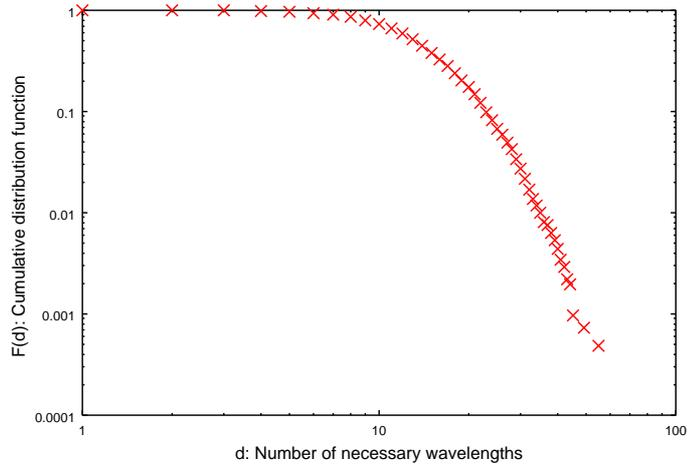
Figure 9: Distribution of the number of required wavelengths: the ER model with wavelength conversion
