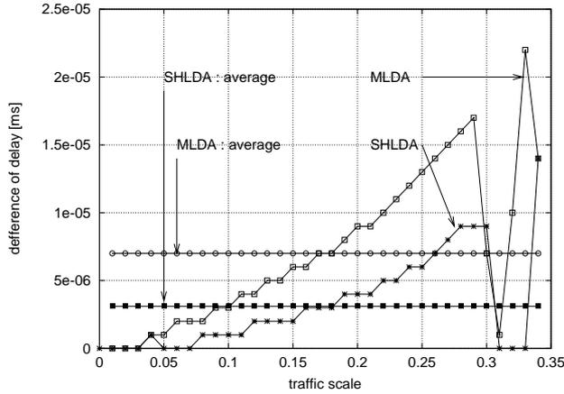
**Fig. 11** Route stability: Delay difference between the first and second shortest path ( $W = 8$ ,  $\mu = 40$  Mpps)
