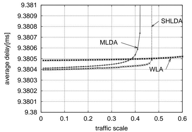
Fig. 10 Average delay of end-to-end paths:  $W = 12, \mu = 100$  Mpps
