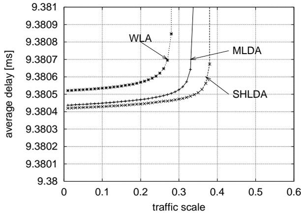
Fig. 7 Average delay of end-to-end paths:  $W = 12, \mu = 40$  Mpps
