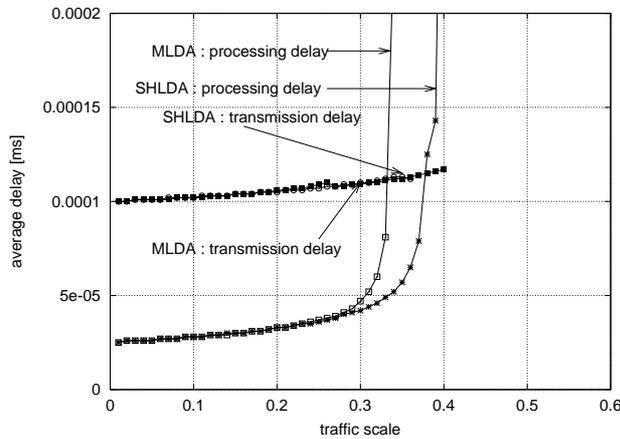
Fig. 8 Average of packet processing and transmission delays at electronic routers:  $W = 12, \mu = 40$  Mpps
