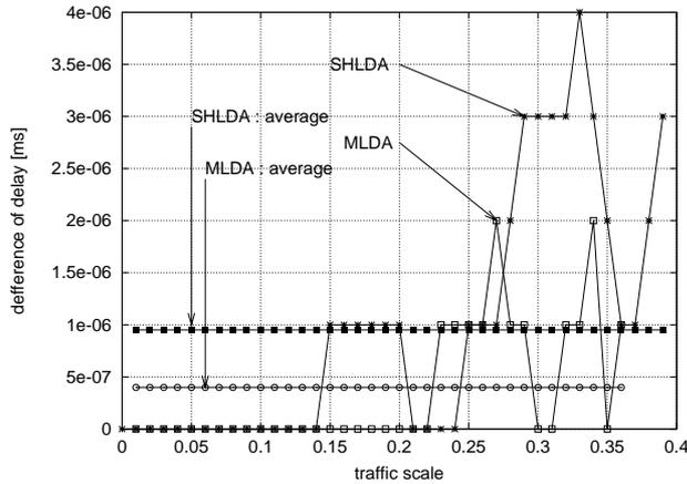
**Fig. 12** Route stability: Delay difference between the first and second shortest path ( $W = 12$ ,  $\mu = 40$  Mpps)
