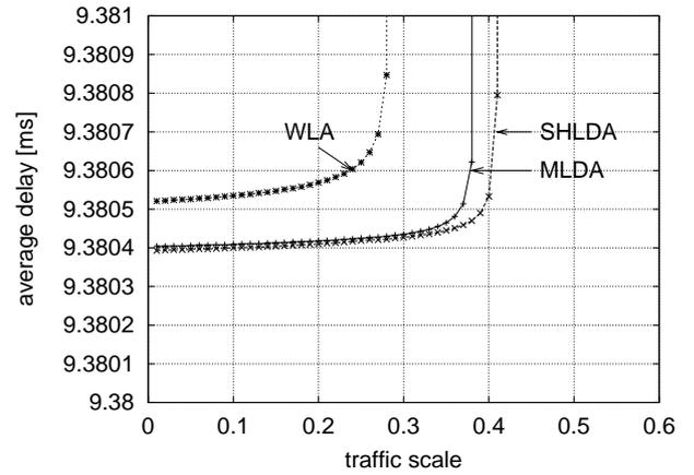
Fig. 9 Average delay of end-to-end paths:  $W = 20, \mu = 40$  Mpps
