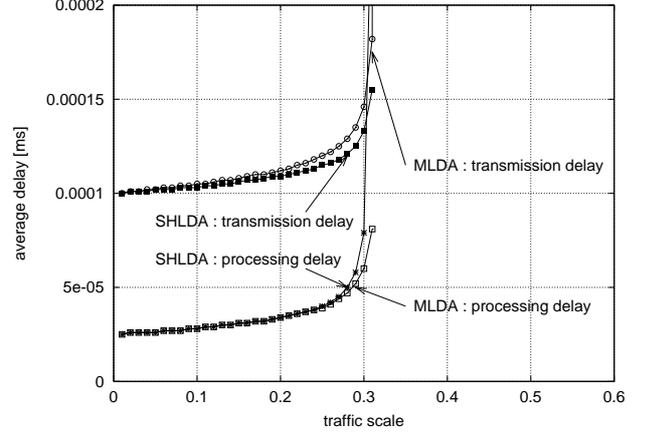
Fig. 5 Average of packet processing and transmission delays at electronic routers :  $W = 8, \mu = 40$  Mpps
