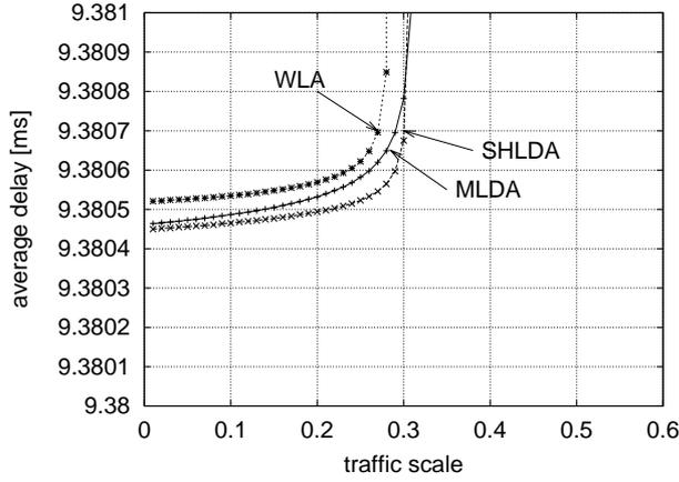
Fig. 3 Average delay of end-to-end paths :  $W = 8, \mu = 40$  Mpps
