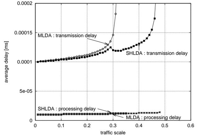
Fig. 6 Average of packet processing and transmission delays at electronic routers:  $W = 8, \mu = 100$  Mpps
