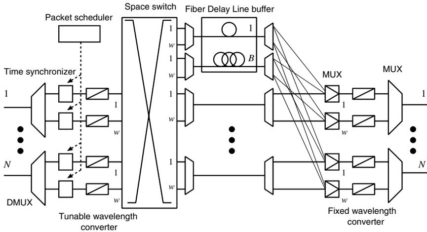
Fig. 3 Shared buffer type photonic packet switch architecture
