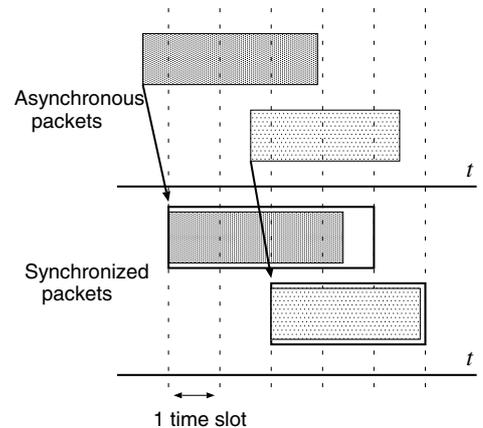
Fig. 1 Synchronization of packets inside a switch
