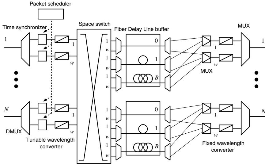
Fig. 2 Output buffer type photonic packet switch architecture
