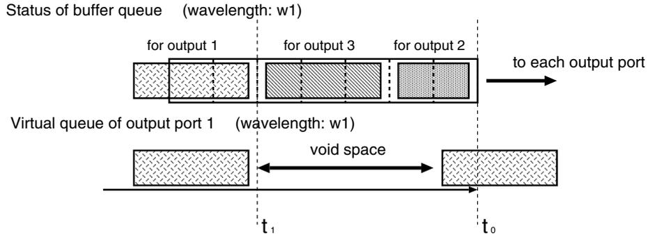
Fig. 4 Void space in shared buffer type switch
