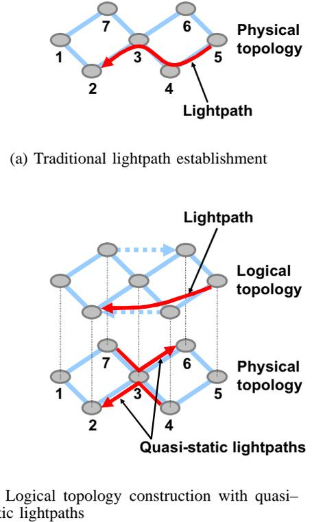
Fig. 6. Concept of quasi-static lightpath (The links without arrows are bi-directional.)
