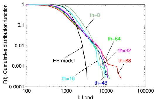
Fig. 11. Distributions of link loads distances between nodes on logical topologies
