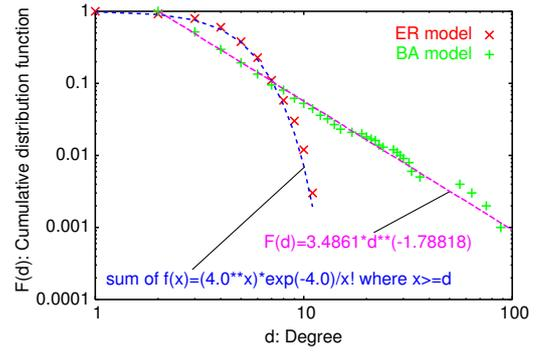
Fig. 2. Cumulative distribution functions of node degrees in topologies generated with the ER and BA models
