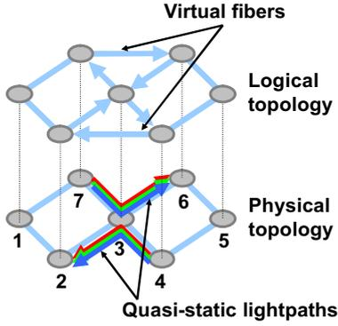
Fig. 7. Concept of virtual fiber (The not arrow links are bi-directional.)
