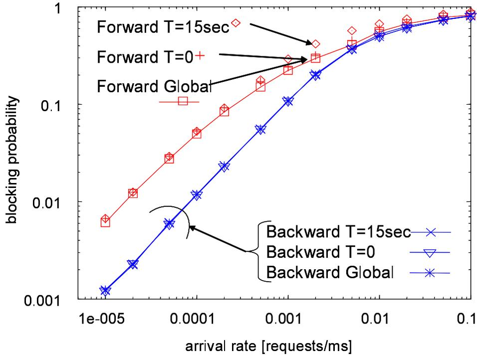
Figure 10: Blocking probability and link state update interval in Japan backbone network:  $W = 8$ ,  $1/\mu = 1\text{ms}$ , average link propagation delay of 0.59 ms
