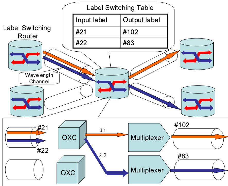
Figure 3: GMPLS label switched lightpath network
