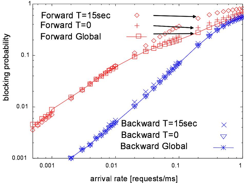
Figure 8: Blocking probability and link state update interval in random network :  $W = 8$ ,  $1/\mu = 1.0\text{ms}$ , average link propagation delay of  $0.1\text{ms}$  ( $\alpha = 0.0557\text{ms}$ )
