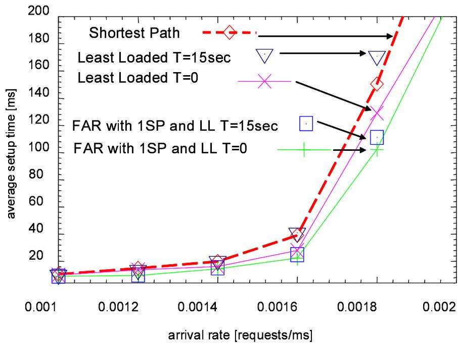
Figure 15: Average path setup time for Japan backbone network with periodic link use information:  $W = 8$ ,  $1/\mu = 1.0\text{ms}$ .
