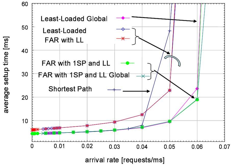
Figure 12: Average path setup time for random network with dynamic link use information:  $W = 8$ ,  $1/\mu = 1.0\text{ms}$ , average link propagation delay of  $0.1\text{ ms}$
