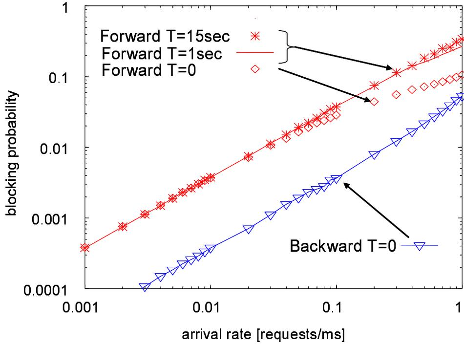
Figure 11: Blocking probability in three node tandem network  $W = 8$ ,  $1/\mu = 1.0\text{ms}$ , average link propagation delay of  $0.1\text{ms}$
