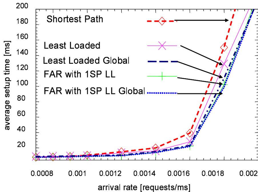
Figure 14: Average path setup time for Japan backbone network with dynamic link use information:  $W = 8$ ,  $1/\mu = 1.0\text{ms}$
