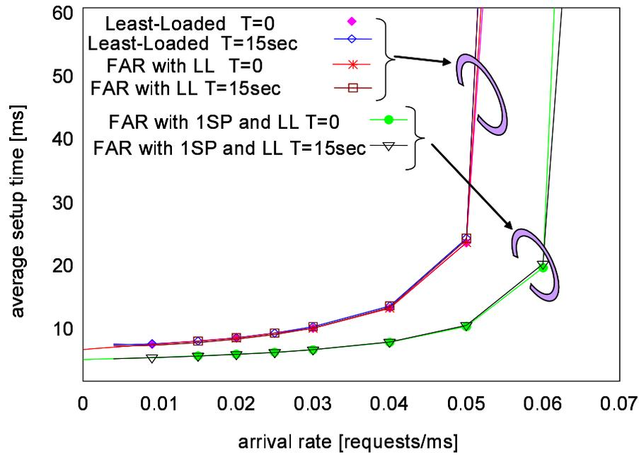
Figure 13: Average path setup time for random network with periodic link use information:  $W = 8$ ,  $1/\mu = 1.0\text{ms}$ , average link propagation delay of  $0.1\text{ms}$
