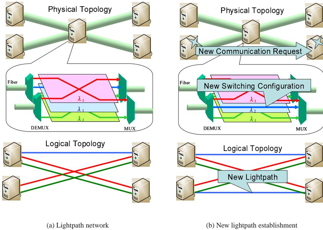
Figure 1: Lightpath network: physical topology, logical topology, and switching
