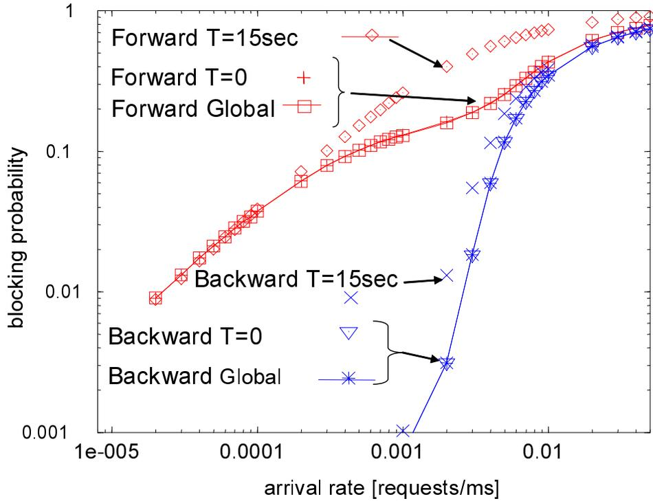
Figure 9: Blocking probability and link state update interval in random network :  $W = 8$ ,  $1/\mu = 100\text{ms}$ , average link propagation delay of  $0.1 \text{ ms}$  ( $\alpha = 0.0557\text{ms}$ )
