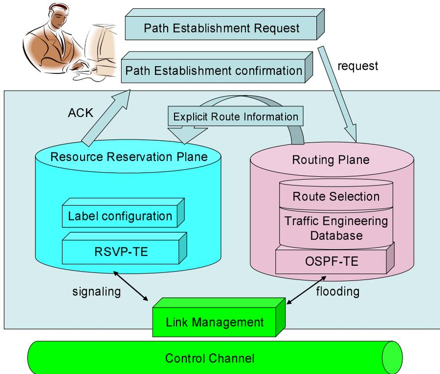
Figure 16: GMPLS signaling architecture and its control plane
