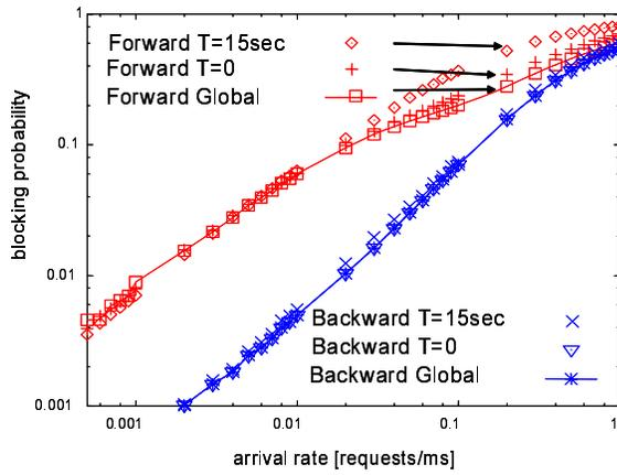
Fig. 7. Blocking probability and link state update interval in random network :  $W = 8$ ,  $1/\mu = 1.0\text{ms}$ , average link propagation delay of  $0.1\text{ms}$  ( $\alpha = 0.0557\text{ms}$ )
