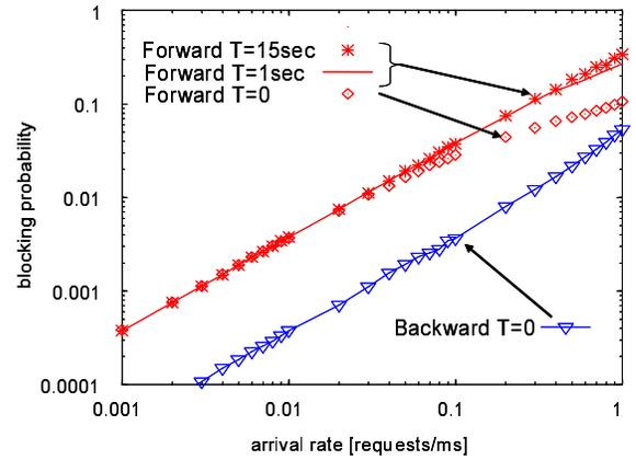
Fig. 10. Blocking probability in three node tandem network  $W = 8$ ,  $1/\mu = 1.0\text{ms}$ , average link propagation delay of  $0.1\text{ms}$
