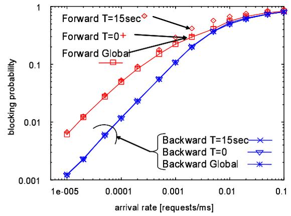
Fig. 9. Blocking probability and link state update interval in Japan backbone network:  $W = 8$ ,  $1/\mu = 1\text{ms}$ , average link propagation delay of  $0.59\text{ms}$
