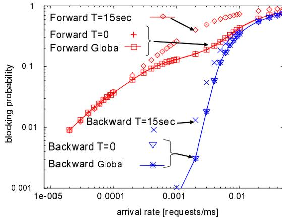
Fig. 8. Blocking probability and link state update interval in random network :  $W = 8$ ,  $1/\mu = 100\text{ms}$ , average link propagation delay of  $0.1\text{ms}$  ( $\alpha = 0.0557\text{ms}$ )
