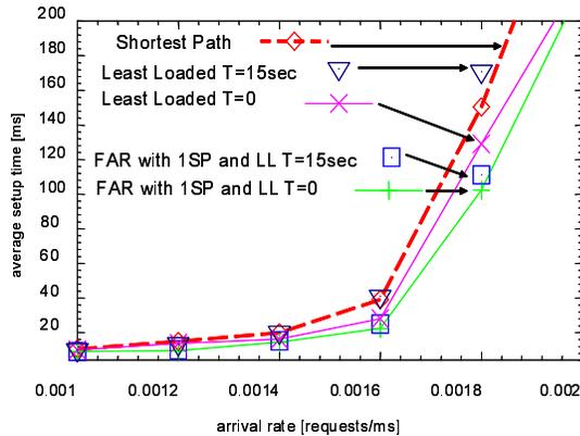
Fig. 14. Average path setup time for Japan backbone network with periodic link use information:  $W = 8$ ,  $1/\mu = 1.0\text{ms}$ .
