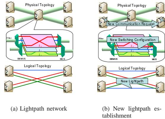
Fig. 1. Lightpath network: physical topology, logical topology, and switching
