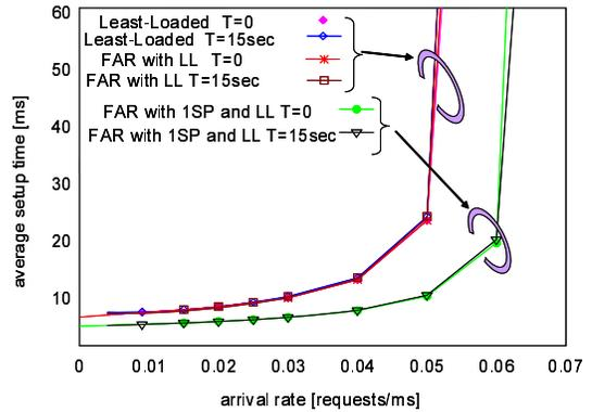
Fig. 12. Average path setup time for random network with periodic link use information:  $W = 8$ ,  $1/\mu = 1.0\text{ms}$ , average link propagation delay of 0.1ms
