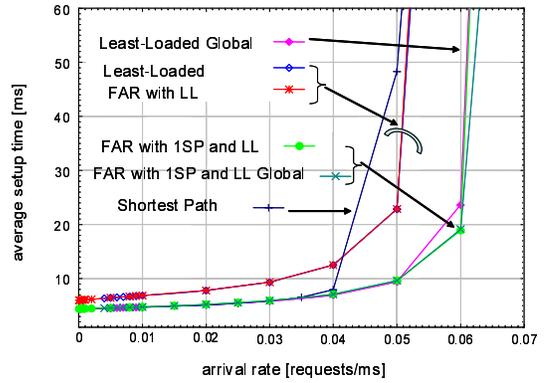
Fig. 11. Average path setup time for random network with dynamic link use information:  $W = 8$ ,  $1/\mu = 1.0\text{ms}$ , average link propagation delay of 0.1 ms
