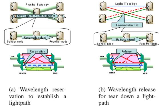
Fig. 2. Lightpath establishment and release
