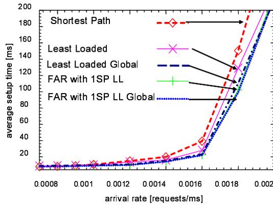
Fig. 13. Average path setup time for Japan backbone network with dynamic link use information:  $W = 8$ ,  $1/\mu = 1.0\text{ms}$
