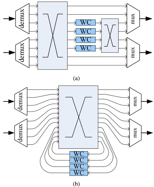
Fig. 1. Node architectures for partial conversion.
