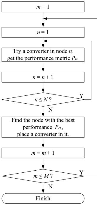
Fig. 2. Heuristic algorithm for converter placement.
