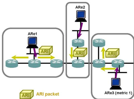
Figure 10: ARIP: Reduce the Time to Converge
