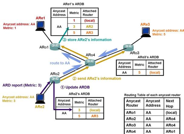
Figure 4: Basic Operation of Advertising Receiver Metric
