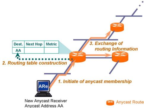
Figure 3: Overview of Anycast Routing Protocol
