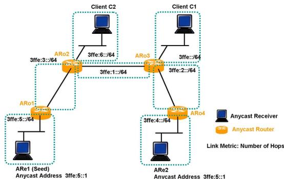
Figure 9: Environment for Experiment
