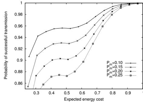
Fig. 2. Probability of successful packet transmission over a path versus its energy cost. Curves are displayed for various maximum link error rates  $P_m$ .
