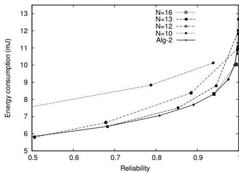
Fig. 7. Comparison between the performance of the energy-reliability trade-off algorithm Alg-2 (the bottom curve) with that of algorithm Alg-1, for which the number of data packets  $N$  is fixed. Curves of algorithm Alg-1 are displayed for various values of  $N$ . These results are generated with  $K=4$  and  $a=8$ .
