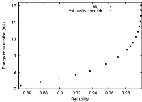
Fig. 3. Comparison between the performance of the path allocation algorithm Alg-1 with that of exhaustive search for a fixed number of data packets  $N = 20$ .
