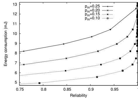
Fig. 6. Performance of the transmission schemes generated by the energy-reliability trade-off algorithm Alg-2 for various maximum link error rates.
