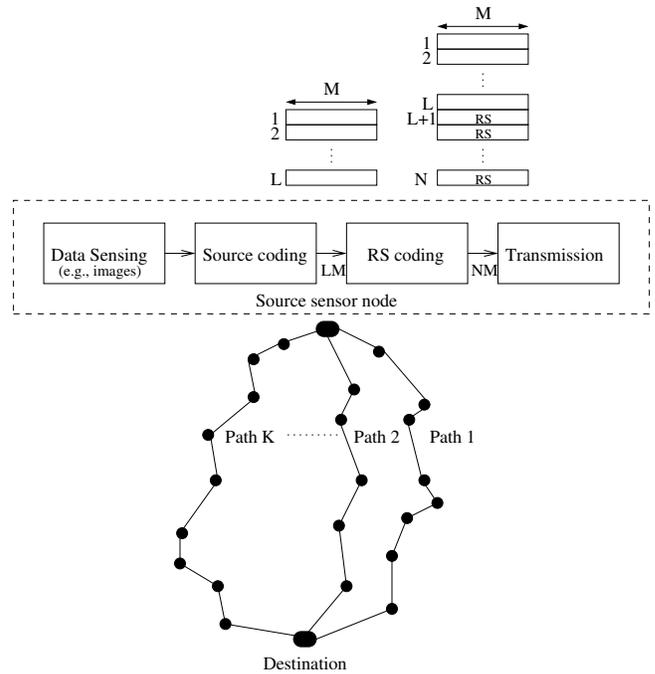
Fig. 1. Block diagram of the reliable multi-path transmission mechanism. A Reed-Solomon (RS) coder appends a number of redundancy packets to the  $L$  information packets. The resulting  $N$  data packets are then transmitted over the  $K$  paths to the destination.
