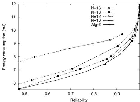
Fig. 4. Comparison between the performance of the energy-reliability trade-off algorithm Alg-2 (the bottom curve) with that of algorithm Alg-1, for which the number of data packets  $N$  is fixed. Curves of algorithm Alg-1 are displayed for various values of  $N$ .
