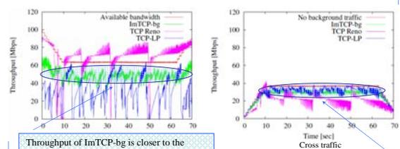
Throughput of ImTCP-bg is closer to the available bandwidth than that of TCP-LP.
