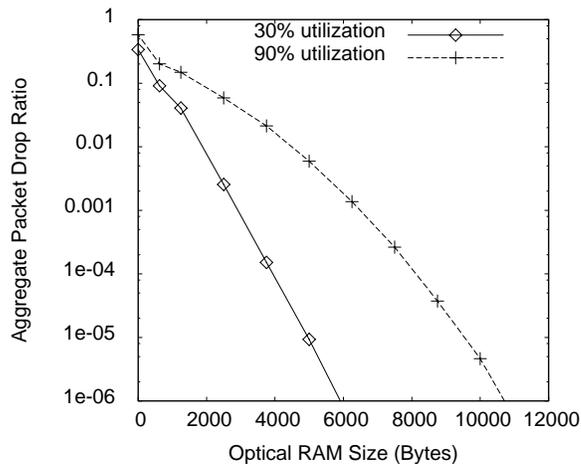
Figure 3. Aggregate packet drop ratio as a function of optical RAM size
