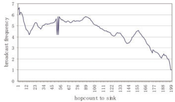
Fig. 5. Average broadcast frequency of individual nodes for 10 000 nodes.
