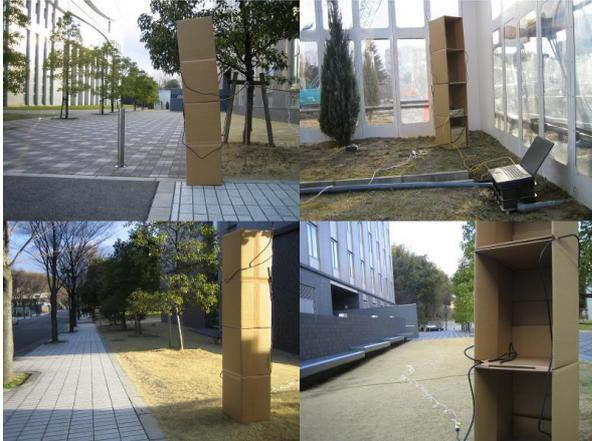
Figure 13: Node placement on practical experiments.
