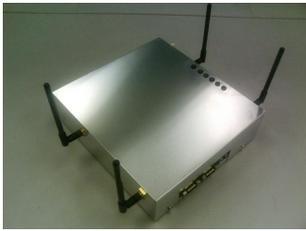
Figure 11: The ad-hoc wireless relay node.
