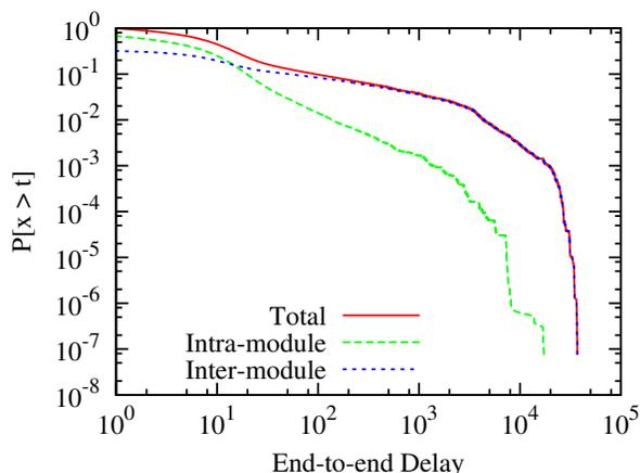
Fig. 6. Comparison of packet delay distribution of intra-module packets and inter-module packets: The number of sessions is 250,000, and data is gathered from  $T = 90,001$  to  $T = 100,000$ . Long-tail distribution is caused by inter-module packets.
