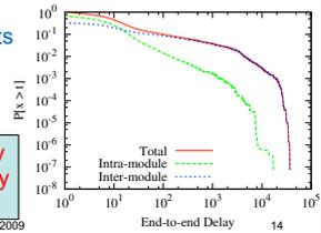
The structure of the AT&T topology lead to this long-tailed packet delay distribution
