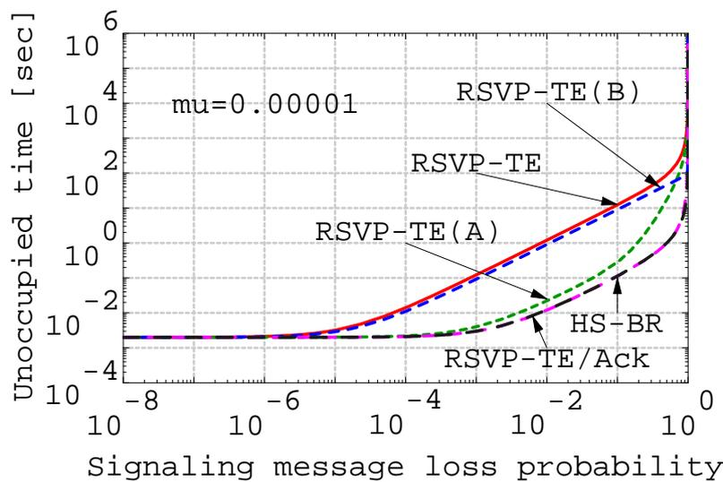
Figure 4. Unoccupied time versus message loss probability for a single-hop LSP without control plane failure
