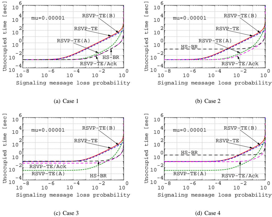
Figure 5. Unoccupied time versus message loss probability for a single-hop LSP with control plane failure
