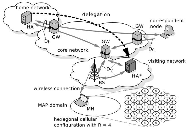
Fig. 1 Mobility model network configuration
