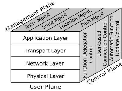
Fig. 5 Layered structure of function-distributed mobility
