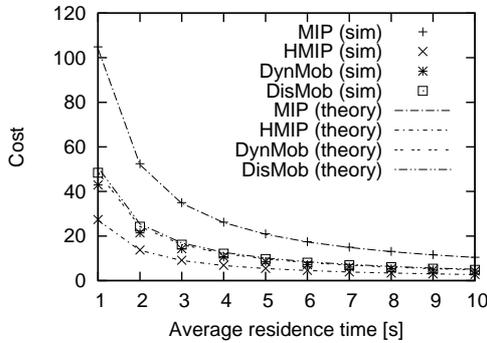
(b)  $R = 4$
