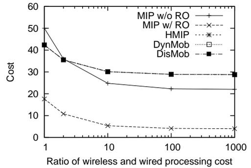
(b)  $R = 4$ **Fig. 6** Location update cost over residence time**Fig. 7** Packet delivery cost over wireless and wired processing cost ratio
