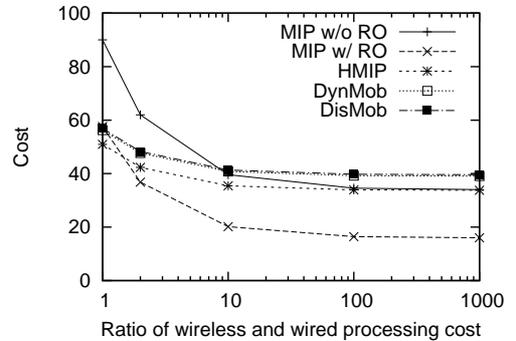
(b)  $R = 4$ **Fig. 10** Total cost over wireless/wired processing cost ratio
