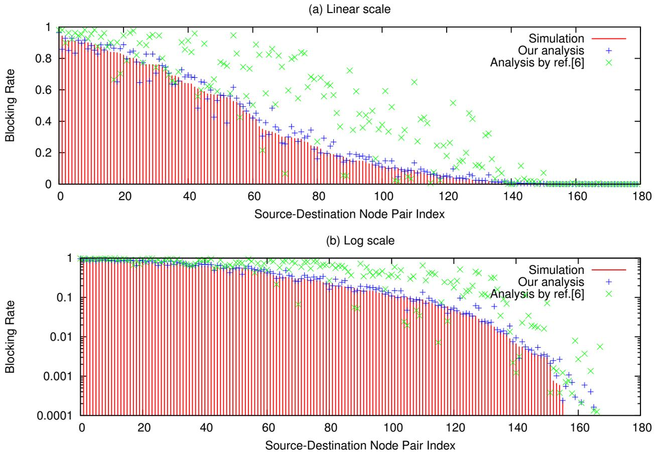
Fig. 4. Comparison of analytical and simulation results when the total reservation request arrival rate in the network is 2000 requests/second
