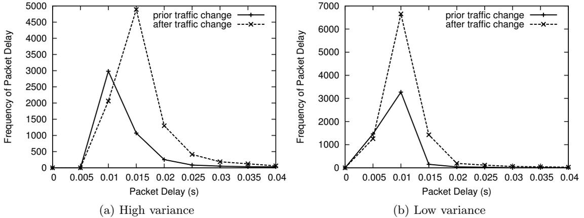
Figure 3.3: Histogram of packet delays when doubling the traffic rate at 500s
