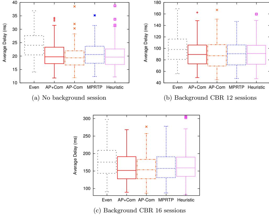
Figure 3.7: Average delay comparison under mobility scenario (y-axis is capped for visibility)
