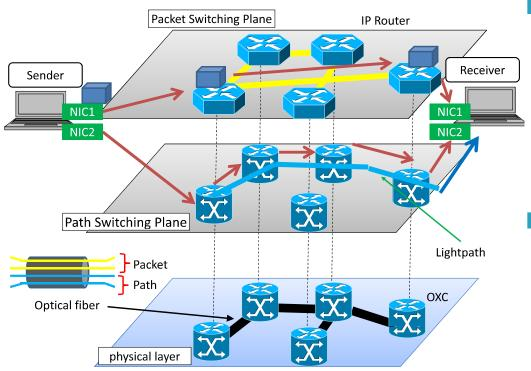
Each end-host connecting with the router has two network interfaces; one for inject IP packets into the packet switched network and one for establish a lightpath between two end-hosts.
