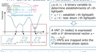
Drive the system with attractor selection and configure a VNT corresponding to the current system state  $x = (x_1, ..., x_{N2})$ .
