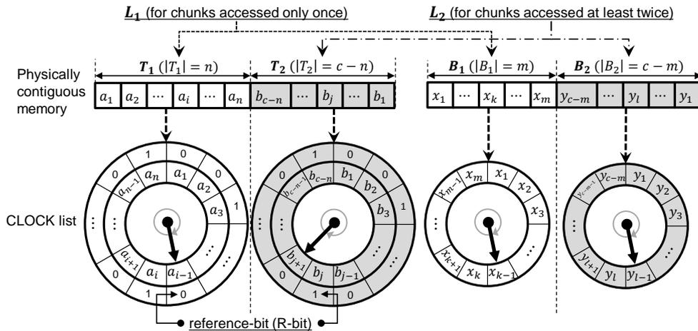
Figure 1. Data Structure of Compact CAR
