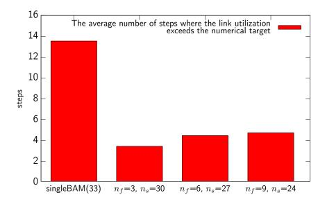
Figure 15: Average number of steps where the link utilization exceeds the threshold: 12-node network
