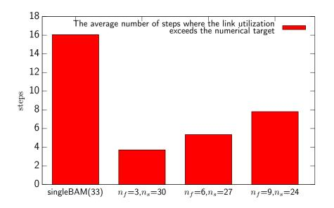
Figure 22: Average number of steps where the link utilization exceeds the threshold: 19-node network
