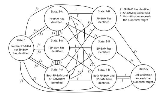
Figure 4: State transition diagram of VNT control using two-pathway BAM
