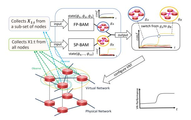
Figure 3: VN Reconfiguration method using two-pathway BAM
