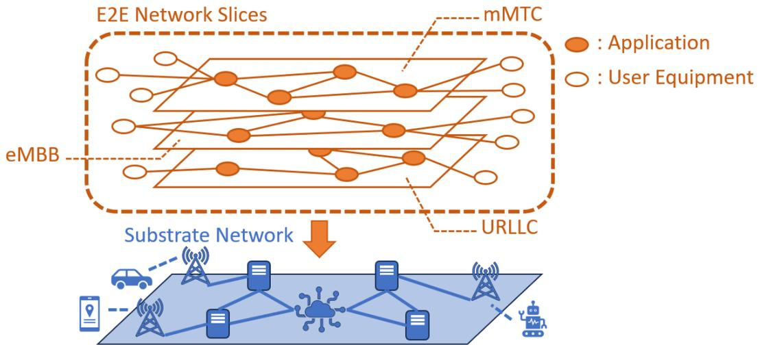
Figure 1: Diagram of E2E network slicing in 5G network
