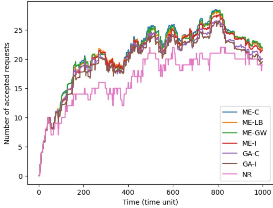
Figure 7: The transition of the number of accepted network slices over time in scenario 1
