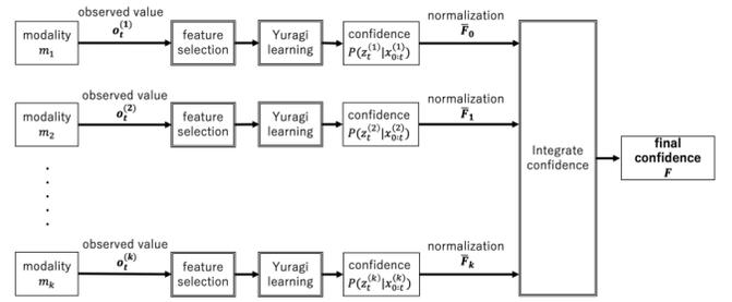
Fig. 2. Stress estimation model of the proposed method
