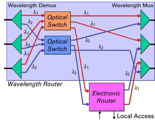
Fig. 9: Structure of wavelength router [62].
