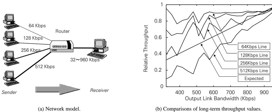
Fig. 7: Comparisons of long-term throughput values of TCP connections with different values of access link capacities.
