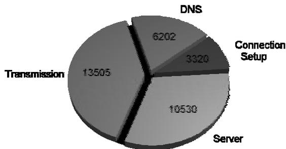
Fig. 4: Delay components of the Web document download. The values in the figure show the 95 percentile delay in milliseconds from randomly chosen 100 sites.
