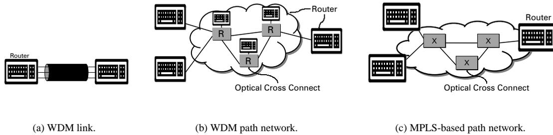
Fig. 8: Structures for IP over WDM networks
