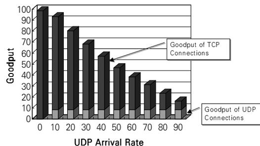
Fig. 5: UDP connections wastes the link and TCP connections receive unfair treatment.
