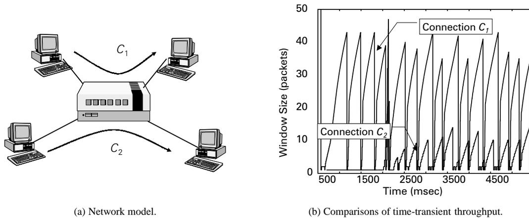
Fig. 6: Comparisons of instantaneous throughput values of TCP connections with different propagation delays. The propagation delay of connection  $C_2$  has two time larger than that of connection  $C_1$ .
