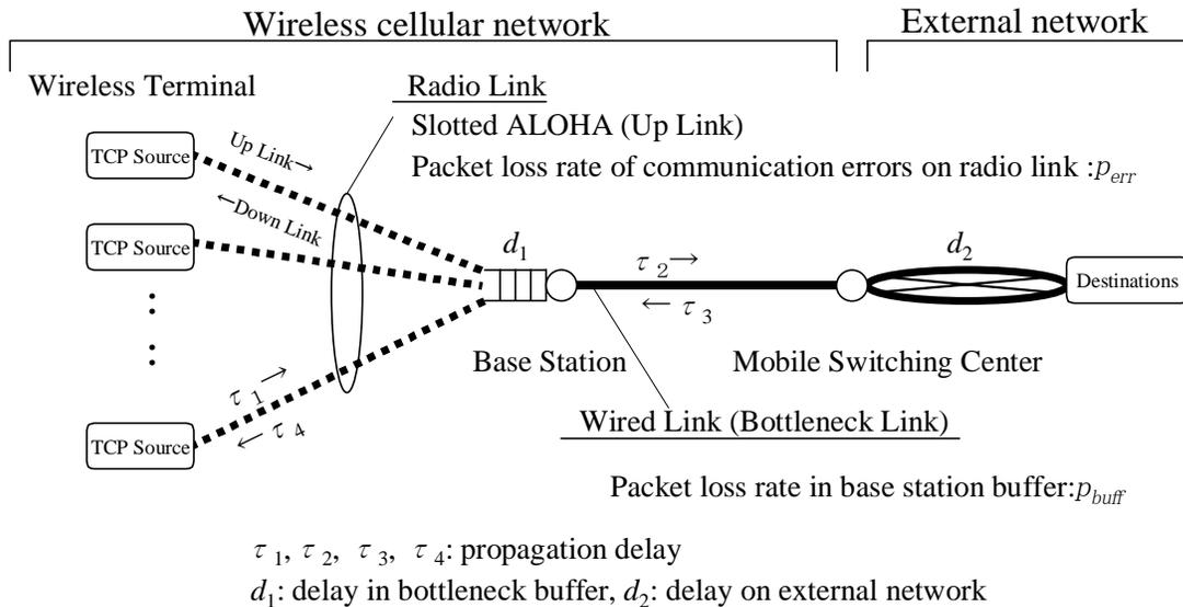
Figure 1: Wireless cellular network model
