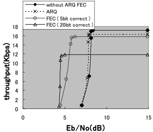
Figure 8: TCP throughput using ARQ, FEC
