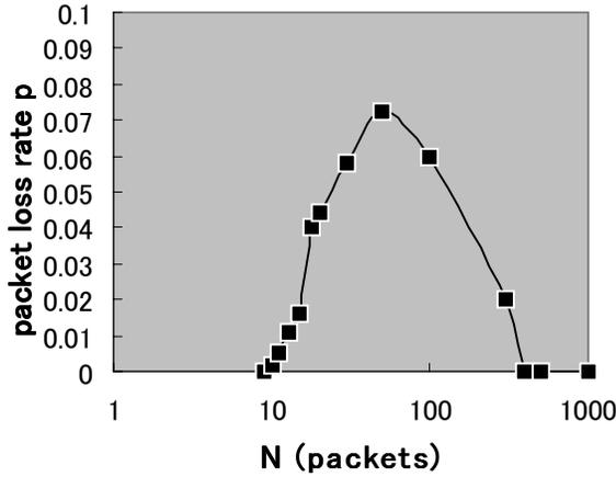
Figure 6: Packet loss rate in BS buffer
