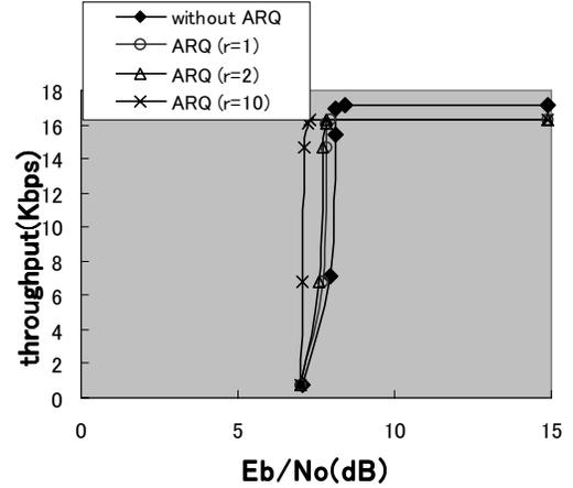
Figure 7: Influences of the number of packet retransmissions on TCP throughput
