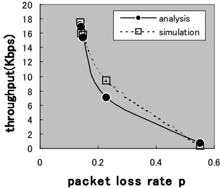
Figure 2: Comparisons of TCP throughput (The number of wireless terminals is 5)
