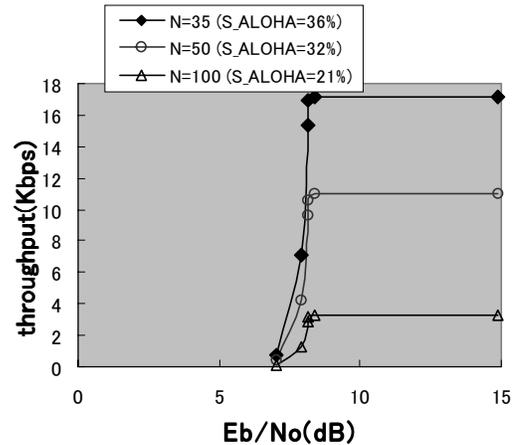
Figure 9: Influences of data link layer throughput on TCP throughput
