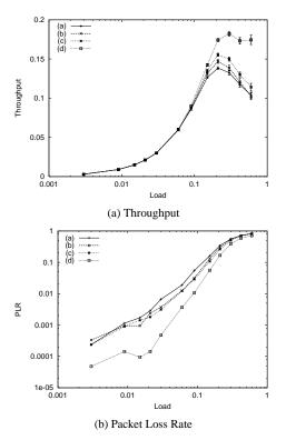
Figure 8: Performance variation by different network configurations
