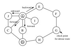
Figure 3: Selection of route for retransmission
