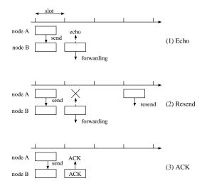
Figure 2: Time chart of packet transmission
